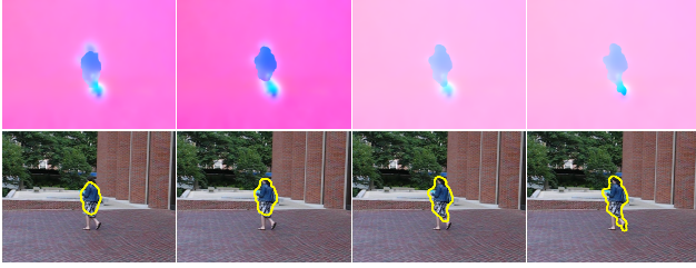
Figure 8. Intermediate steps in the evolution of the velocity (top) and the segmenting curve (bottom) for the motion segmentation based on the global-local tradeoff algorithm.
